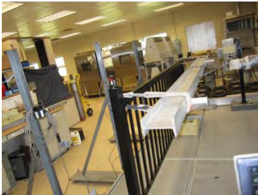
Photo No. 4 Concentrated Load Test at End of Top Rail (Bracket) and Post Tests
