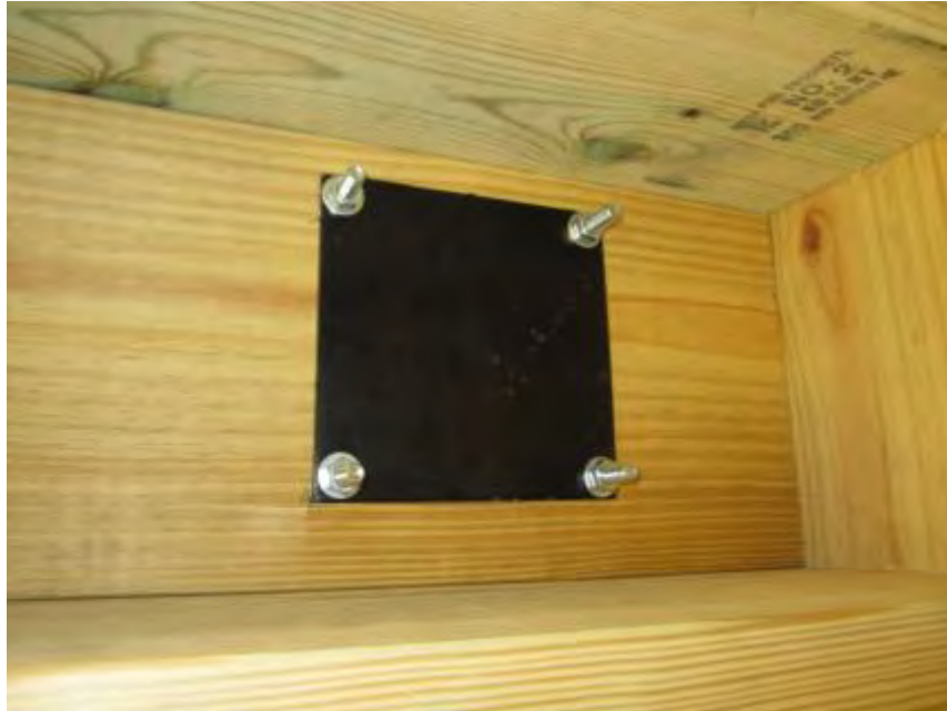
Photo No. 5 Post Mount Attached to Mock Wood Deck
