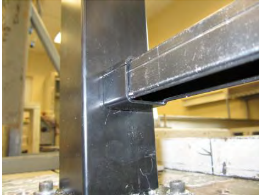
Photo No. 7 Bottom Rail Bracket-to-Rail Connection
