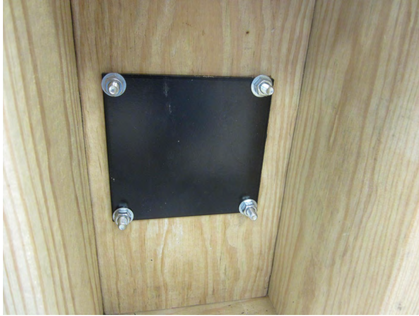
Photo No. 9 3/16 in Thick Mounting Plate Attached to the Underside of the Horizontal Wood Blocking of the Mock Wood Deck
