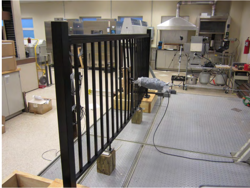
Photo No. 1 Horizontal Infill Test at Center of Three Balusters
