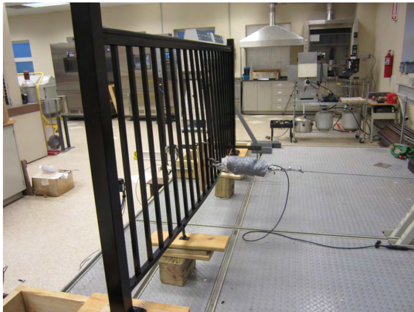
Photo No. 2 Horizontal Infill Test at Bottom of Three Balusters
