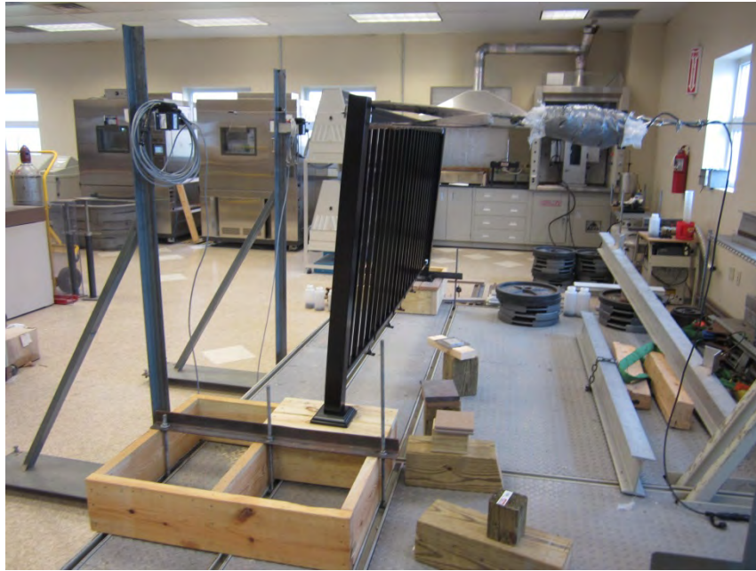
Photo No. 5 Horizontal Concentrated Load Test on Single Post
