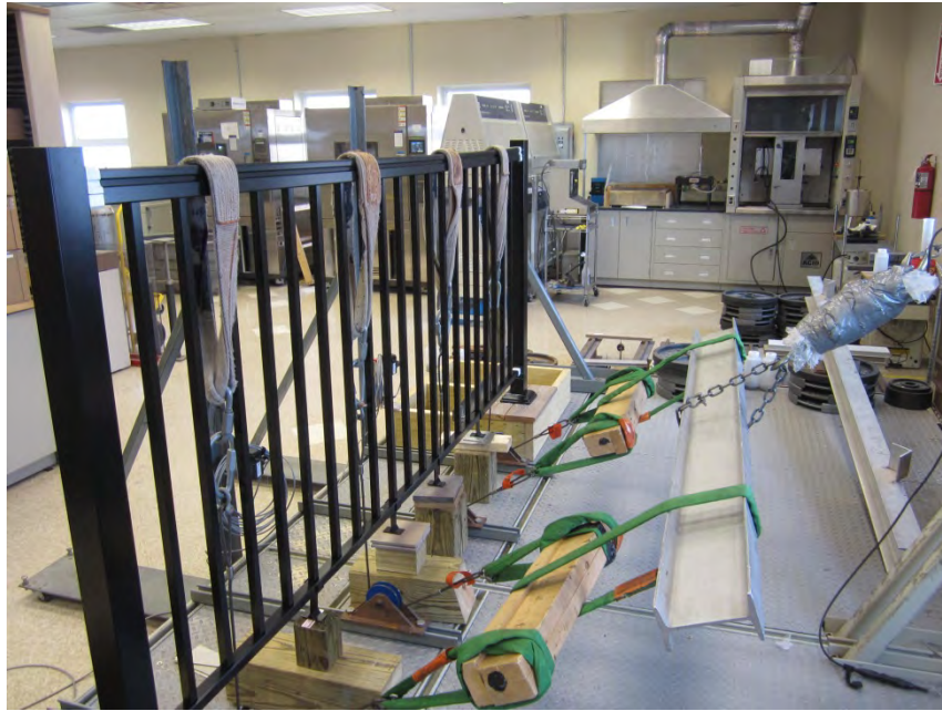
Photo No. 3 Vertical Uniform Load Test
