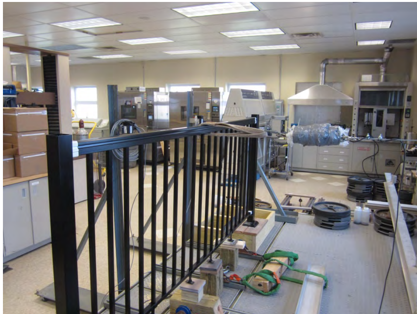
Photo No. 4 Horizontal Concentrated Load at Midspan of Top Rail
