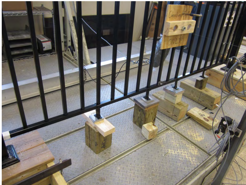
Photo No. 8 Location of Support Blocks Along the Length of the Rail
