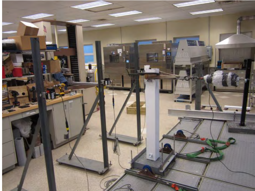
Photo No. 7 Concentrated Load Test at Top of Stand-Alone Post (2 in Square Steel Post Mount with 5 in Square PVC Post Sleeve with Internal Spacers)
