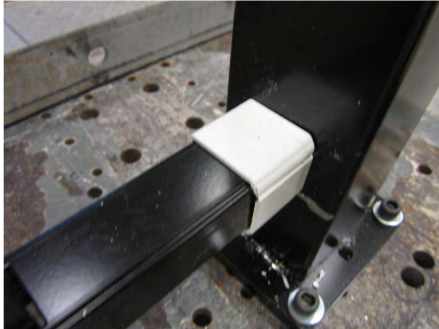
Photo No. 9 Bracket Connection for Bottom Rail
