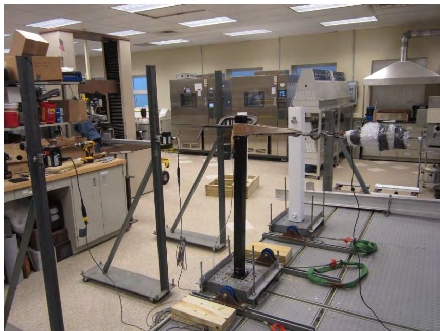
Photo No. 6 Concentrated Load Test at Top of Stand-Alone Post (2 in Square Steel Post Mount with a 2-1/2 in Square Aluminum Post Sleeve)
