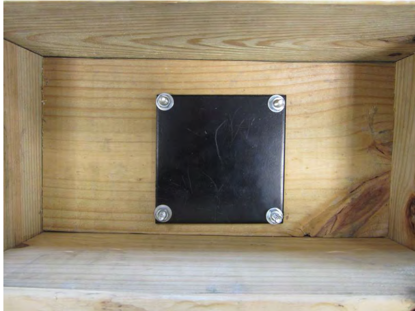
Photo No. 9 Mounting Plate Attachment to the Underside of the Horizontal Wood Blocking of the Mock Wood Deck
