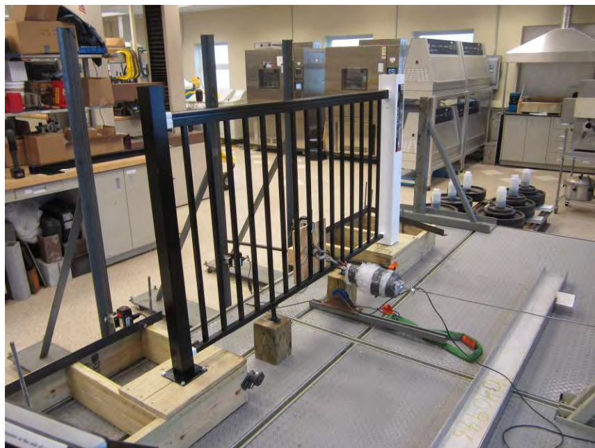
Photo No. 2 Infill Loading at Bottom of Three Balusters
