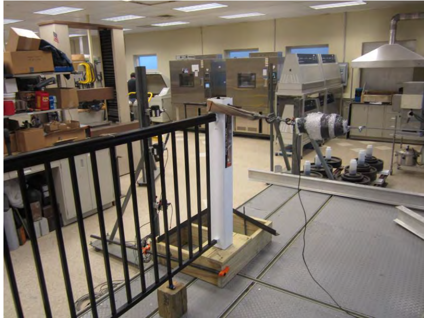
Photo No. 5 Concentrated Load on Top of Single Post
